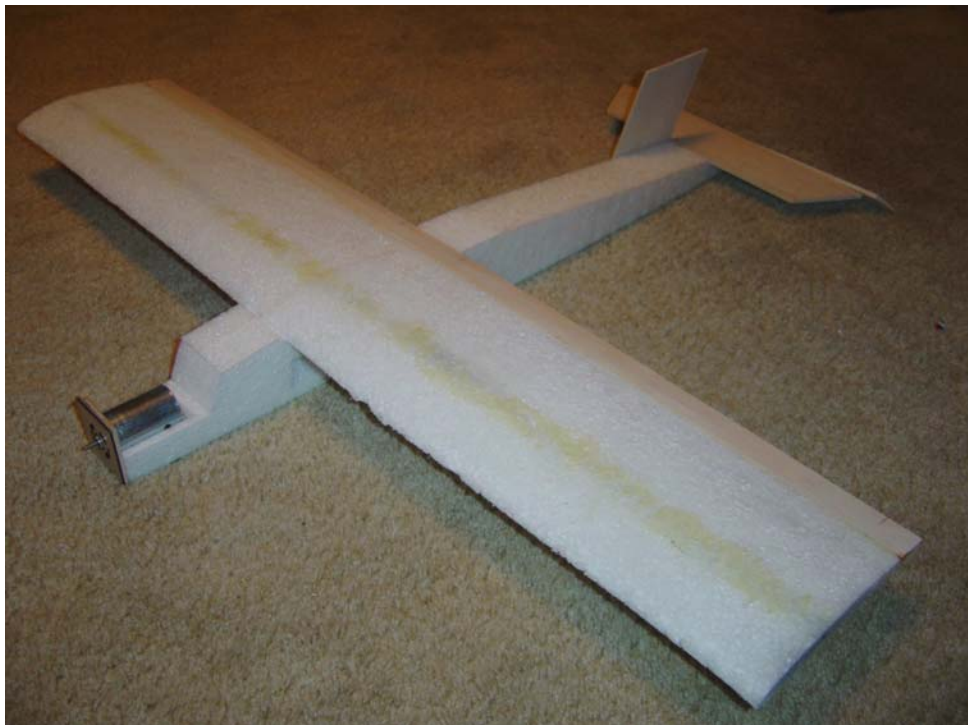
Parts lay out. At this stage, the wing spar, bass wood sub training edge, and tapered trailing edge are installed.
