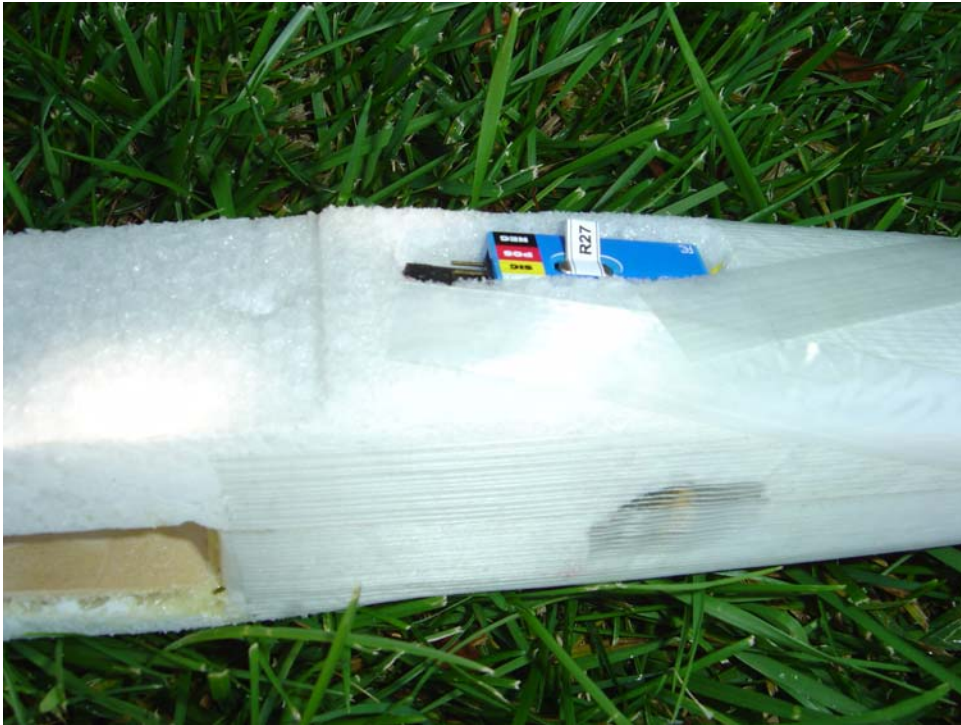
Elevator servo and receiver placement, also note fuse taping and plywood floor for the battery compartment.
