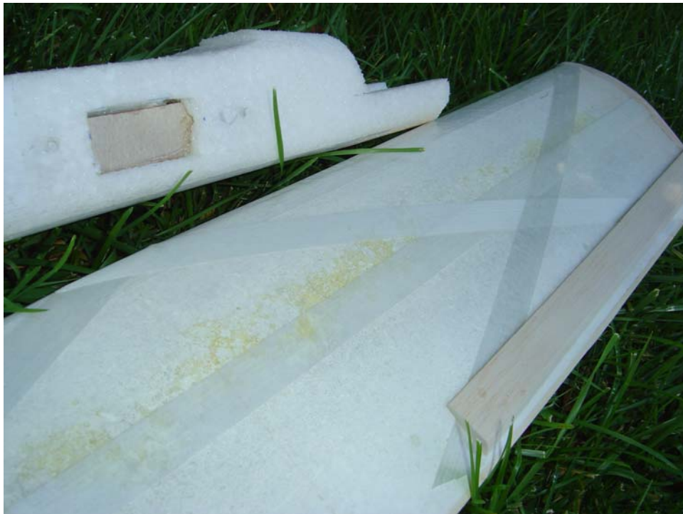
View of the top of the wing showing the taping, and of the right side of the fuselage where the speed controller was mounted. Wing spar was installed using Elmers Pro Bond PU glue.
